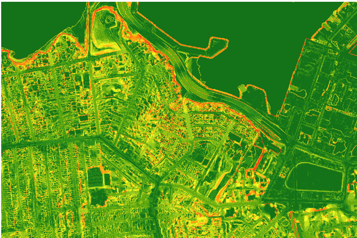
Figure 44: Slope angle raster from the 2016 LIDAR DEM, Freemans Bay, with original DEM using AVD1946 elevations.
