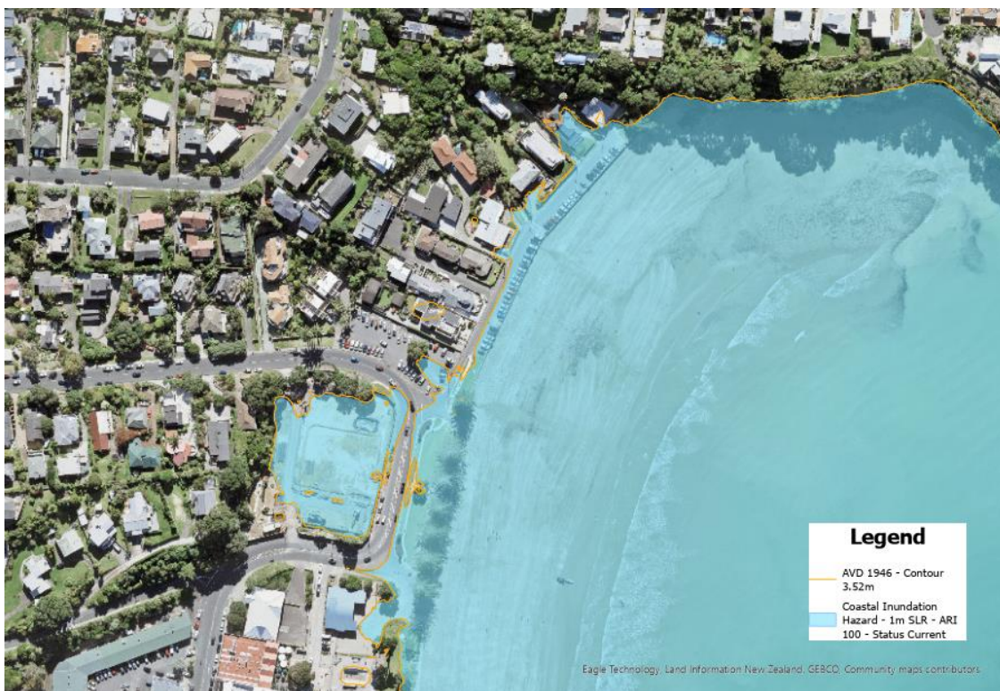
Figure 45: Comparison of ARI 100 inundation zone with 1m SLR (blue) with 3.52m contour based off 2016-2018 DEM in AUK1946 datum (Browns Bay, North Shore)
