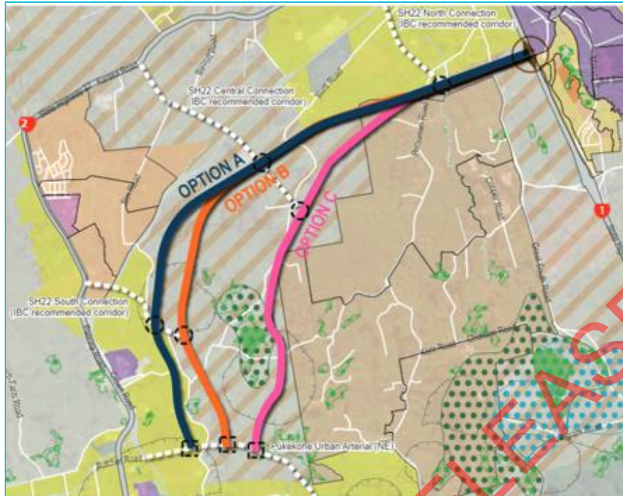
Figure 4-7 Summary of Pukekohe Expressway (B) options (Source: Strategic South Detailed Business Case, July 2020).
