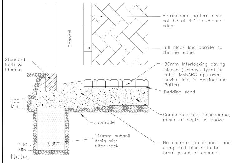
1. Paving blocks, design and construction to be in accordance with NZS 3116.
