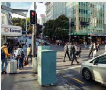
Figure 4 Poor practice Poorly located signal control box that blocks the corner where pedestrians wait to cross the intersection. Fanshawe Street, City Centre.
