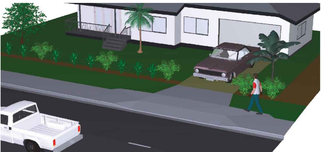
VEHICLE CROSSING WITH FOOTPATH <1.8m
