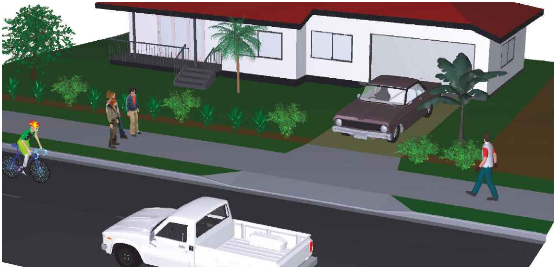
VEHICLE CROSSING FOOTPATH SEPARATED FROM KERB
