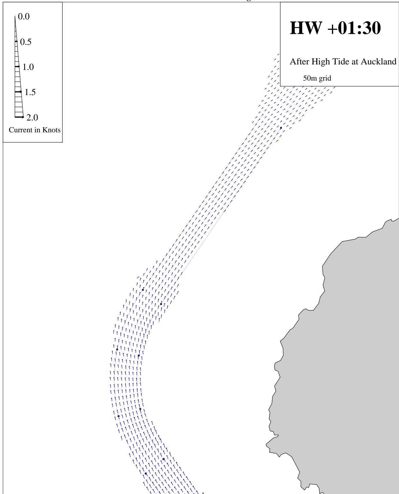
ADCP measured tidal currents for vessel simulator, surveyed 2014 (inner harbour)+2019 (Rangitoto channel)
