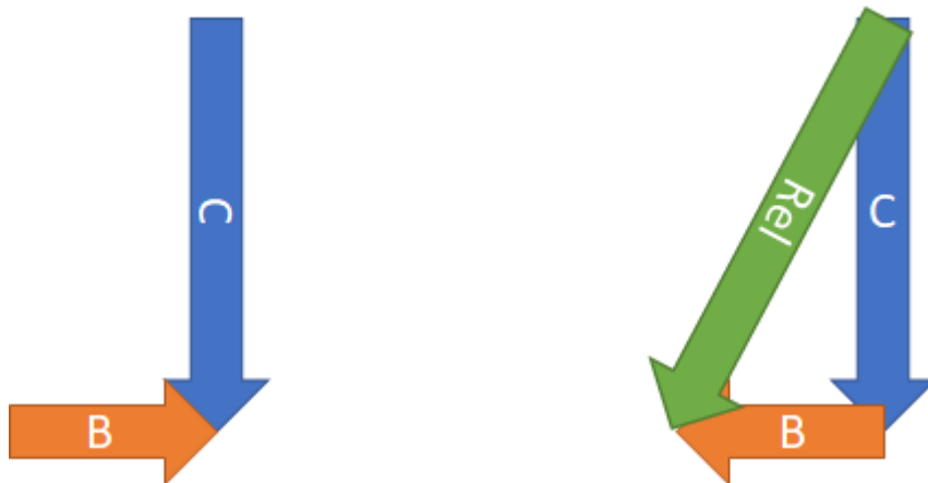
Figure 1(b). Vector diagram of a car striking a cyclist travelling at 25 km/h at right angles at 50 km/h. The magnitude of the cyclist velocity change is 55.9 km/h ( \sqrt{25^2 + 50^2} ).
