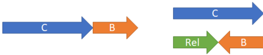
Figure 1(a). Vector diagram of a car striking a cyclist travelling at 25 km/h from behind at 50 km/h. The magnitude of the cyclist velocity change is 25 km/h.
