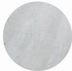
Standard form finish box girder finish.
