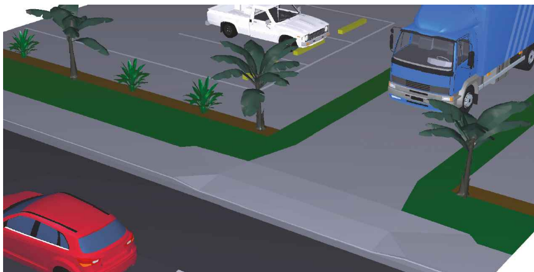
VEHICLE CROSSING WITH FOOTPATH <1.8m
