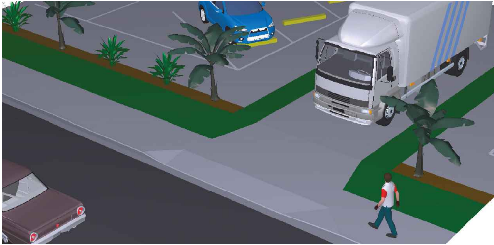
VEHICLE CROSSING FOOTPATH NEXT TO KERB
