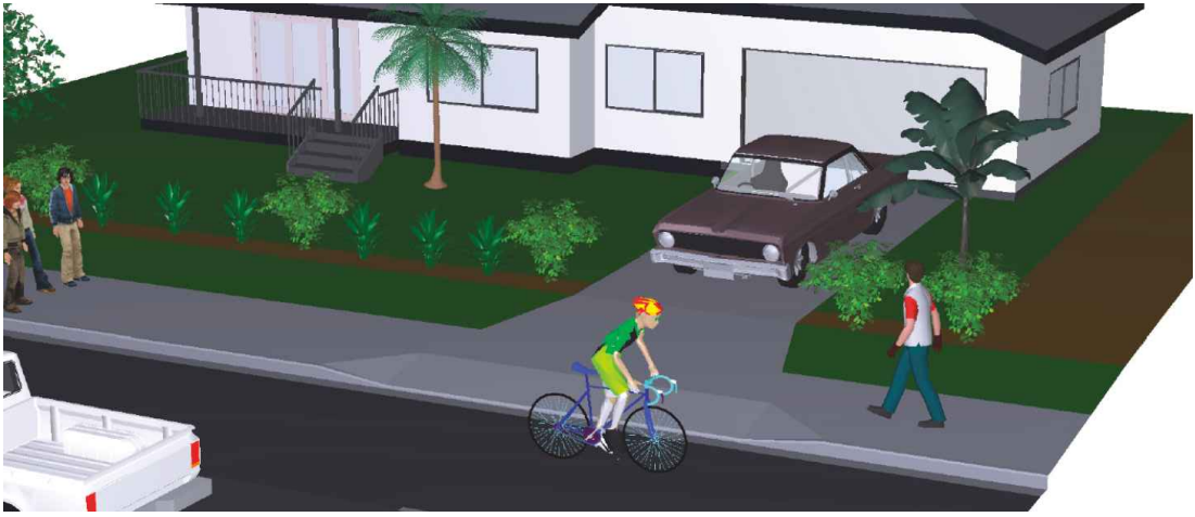
VEHICLE CROSSING FOOTPATH NEXT TO KERB
