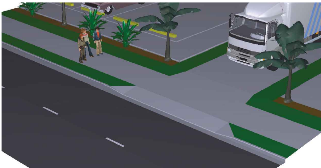
VEHICLE CROSSING FOOTPATH SEPARATED FROM KERB
