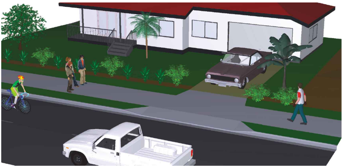
VEHICLE CROSSING FOOTPATH SEPARATED FROM KERB
