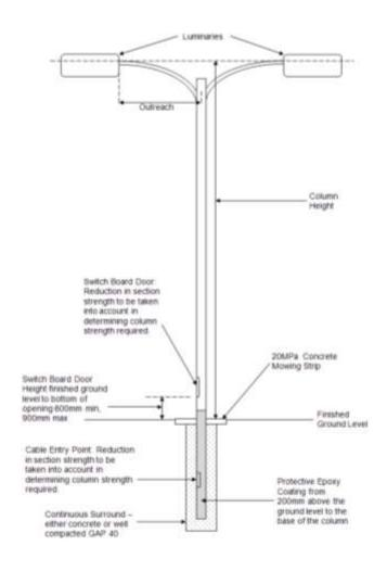
Figure D1: Parts of the lighting column.
