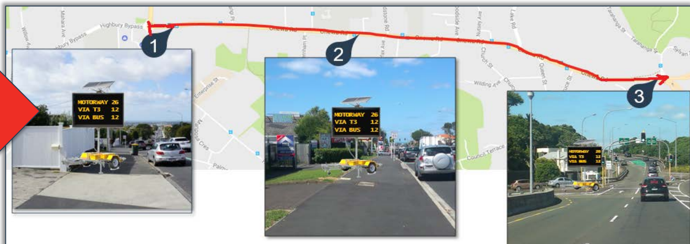
Portable VMS signs were located at three points along Onewa Road
