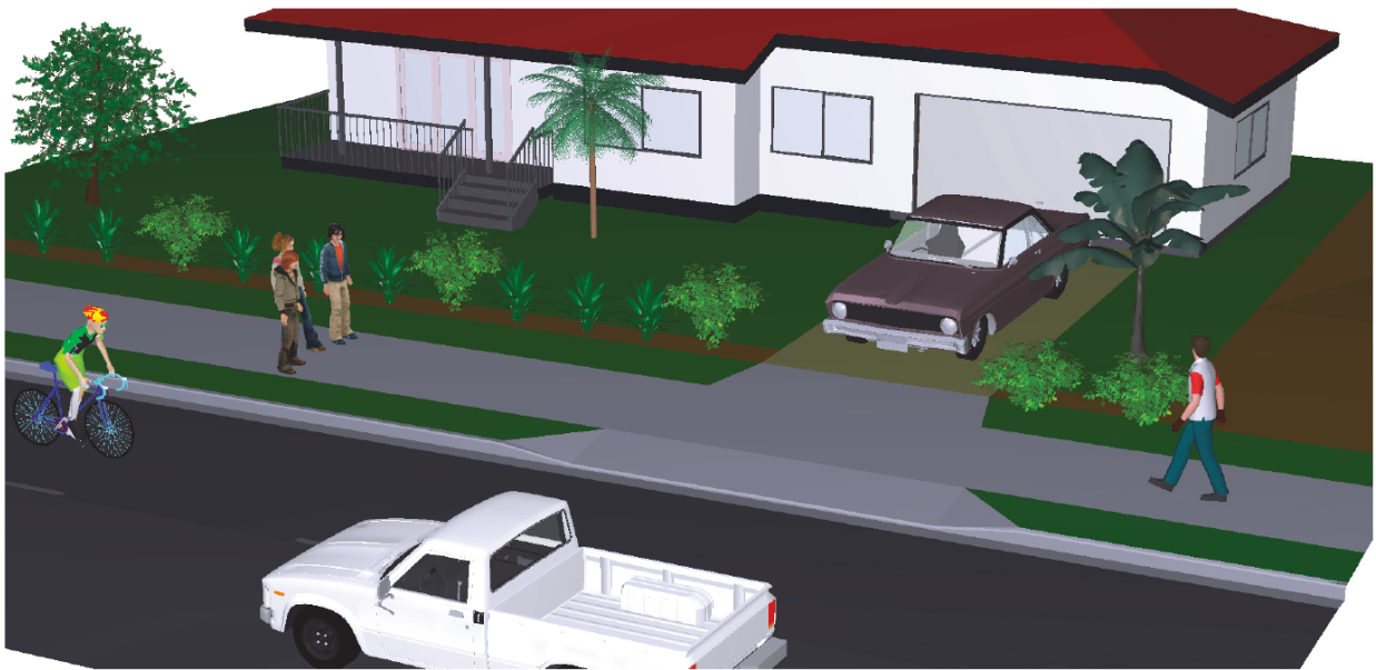
VEHICLE CROSSING FOOTPATH SEPARATED FROM KERB
