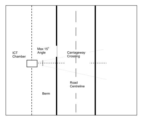
Diagram 8.4.1: Plan of Carriageway Lateral Crossings and Loop Connections
