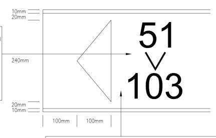
The space from the arrowhead to the first number, either top or bottom is equal to the numeral 5. Numbers are to be central on the vertical plane.
