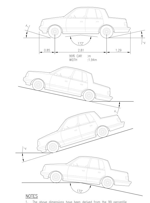
1. The above dimensions have been derived from the 99 percentile car shown in the Auckland City Council District Plan and a road clearance of 100mm as stated in AS2890.1—1993.
