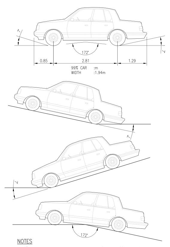
1. The above dimensions have been derived from the 99 percentile car shown in the Auckland City Council District Plan and a road clearance of 100mm as stated in AS2890.1—1993.
